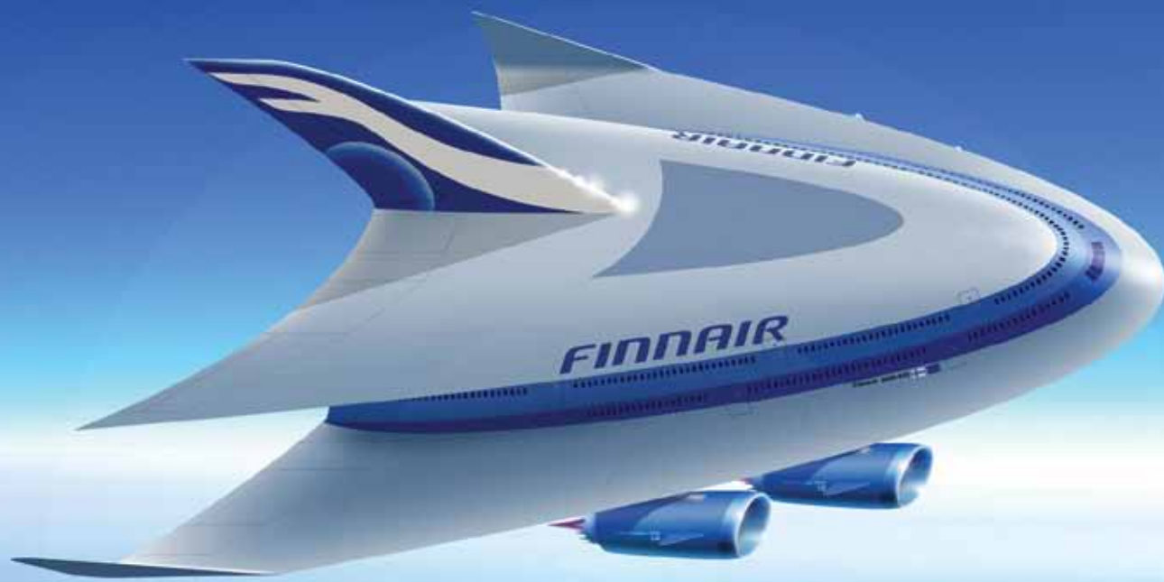
HIGH ON CONCEPT: FINNAIR A600-850 CAN SEAT 600-850 PASSENGERS AND HAS FOUR ENGINES THAT CAN BE TILTED, ALLOWING FOR VERTICAL TAKE-OFFS
