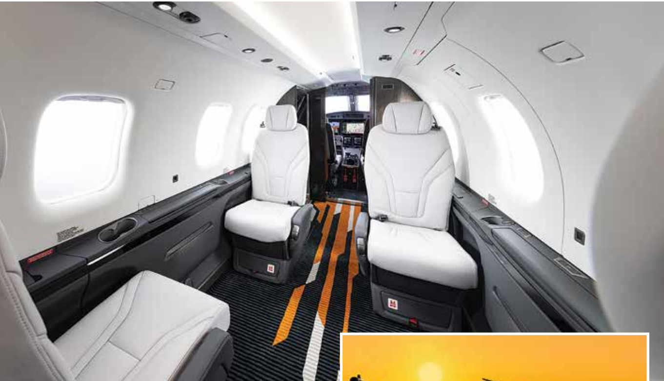
THE LATEST UPGRADE, THE PC-12 PRO, UNVEILED IN 2025, FEATURES GARMIN G3000 PRIME AVIONICS, AUTOLAND, ENHANCED COCKPIT ERGONOMICS, AND READINESS FOR SUSTAINABLE AVIATION FUEL (SAF)
