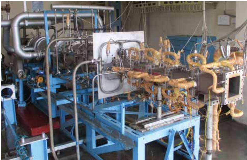
DRDO CONDUCTS LONG-DURATION ACTIVE COOLED SCRAMJET SUBSCALE COMBUSTOR GROUND TESTING. THE DEVELOPMENT OF THIS SCRAMJET ENGINE IS FULLY INDIGENOUS.
