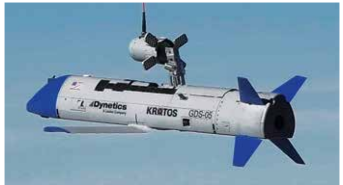
(LEFT) LONGSHOT UNMANNED AIRCRAFT SYSTEM, DROPPED FROM A BOMBER OR FIGHTER THAT CAN LAUNCH MISSILES OF ITS OWN; (RIGHT) X-61 GREMLINS IS A RECOVERABLE, LOW-COST UAV THAT COULD EMPLOY ISR AND OTHER MODULAR, NON-KINETIC PAYLOADS.
