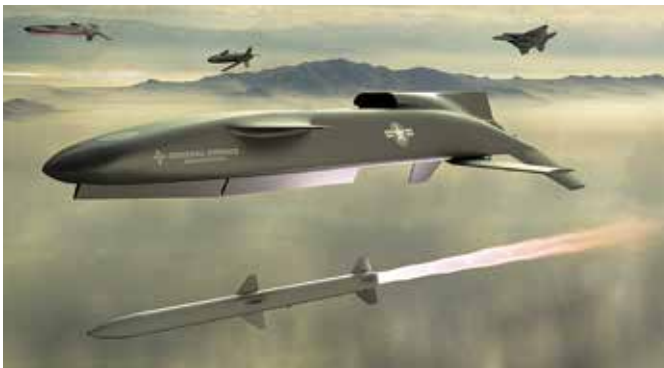
(LEFT) LONGSHOT UNMANNED AIRCRAFT SYSTEM, DROPPED FROM A BOMBER OR FIGHTER THAT CAN LAUNCH MISSILES OF ITS OWN; (RIGHT) X-61 GREMLINS IS A RECOVERABLE, LOW-COST UAV THAT COULD EMPLOY ISR AND OTHER MODULAR, NON-KINETIC PAYLOADS.
