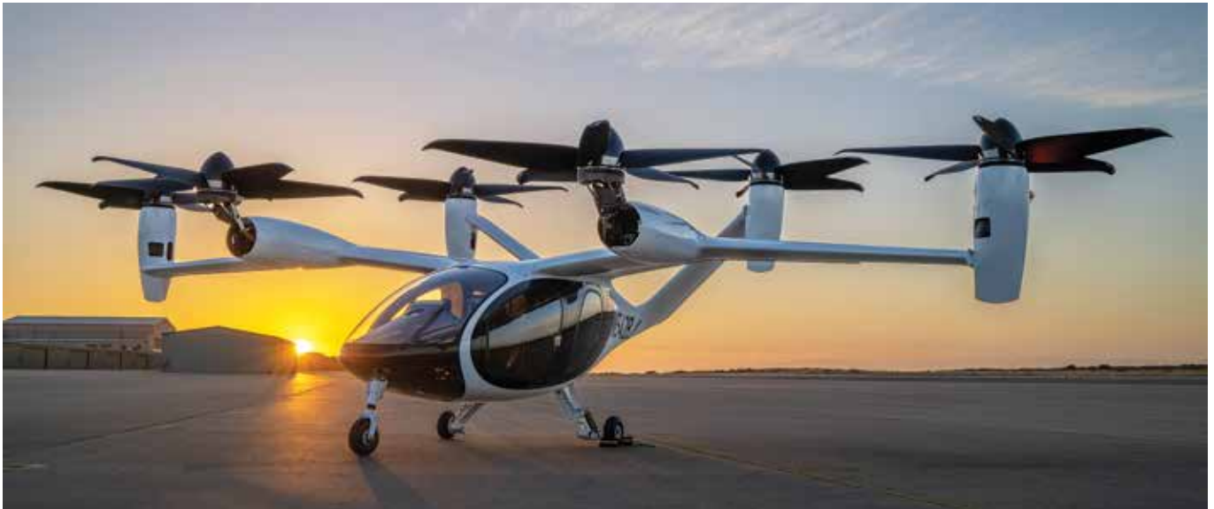
POWERED BY SIX ELECTRIC MOTORS, JOBY'S AIRCRAFT TAKES OFF AND LANDS VERTICALLY SERVING ALMOST ANY COMMUNITY. JOBY BECOMES FIRST EVTOL COMPANY TO SUBMIT AREA-SPECIFIC CERTIFICATION PLAN
