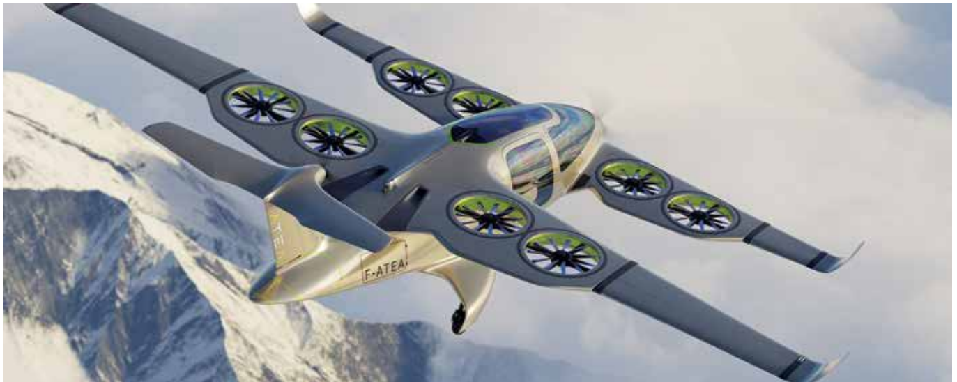
ATEA, A LOW NOISE, LOW CARBON EMISSIONS VTOL AIRCRAFT BY ASCENDANCE IS BASED ON UNIQUE HYBRID PROPULSION TECHNOLOGY
