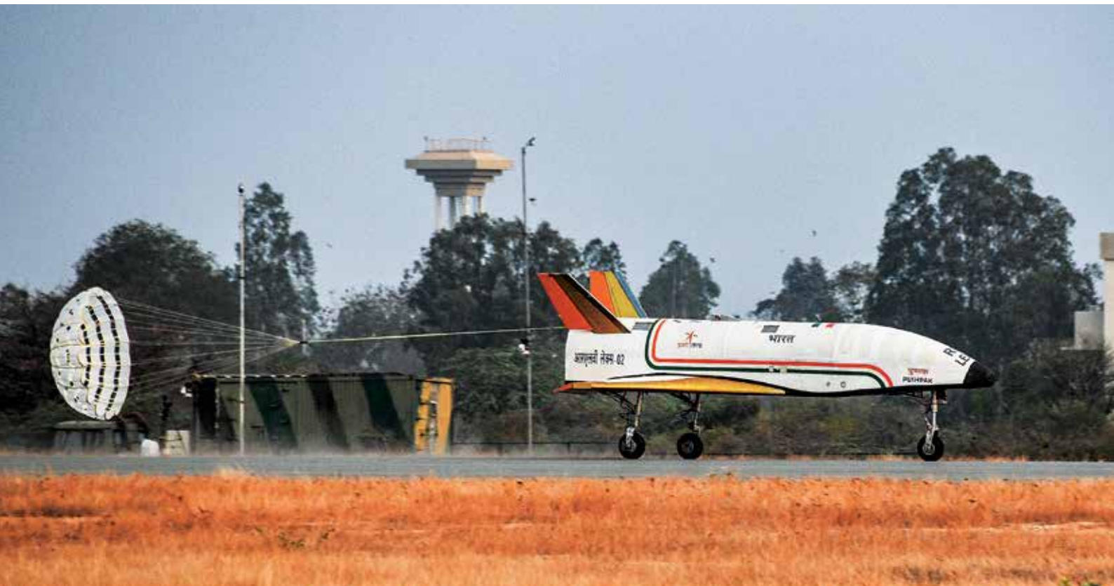
PUSHPAK (RLV-TD), THE WINGED VEHICLE, LANDED AUTONOMOUSLY WITH PRECISION ON THE RUNWAY AFTER BEING RELEASED FROM AN OFF-NOMINAL POSITION
